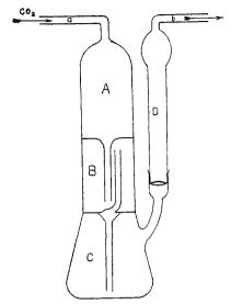
partments B and C contain as much of the solution as would completely fill A, which is about thirty-five to forty grams of a 2:3 solution. D, which is fastened to the bulb by means of a ground-glass joint, contains solid potassium hydroxide, or soda-lime, supported by a plug of glass-wool. The liquids in B and C can be easily mixed when desired, by applying suction at a. The bulb, when filled and ready for use, weighs from sixty-five to seventy grams, and undoubtedly can be made
